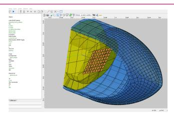
Analyse beam distortion from a phased array through a single- or multilayer radome, and optimise material parameters
