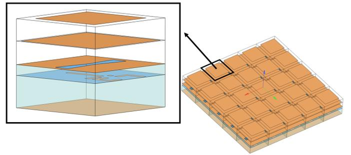
Fig. 3. Simulation model of preliminary reconfigurable array element.
