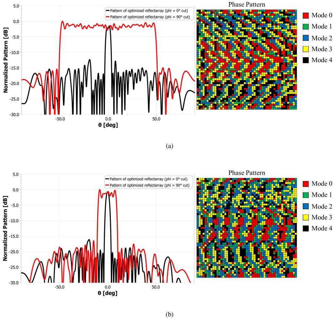
Fig. 9. Far-field radiation pattern of the optimised reflectarray for (a),  $\theta = \pm 50^\circ$  fan beam and (b)  $\theta = \pm 10^\circ$  fan beam. The color codes for the five operating modes over the reflectarray surface is shown together with the radiation pattern. (Optimized for 26 GHz)
