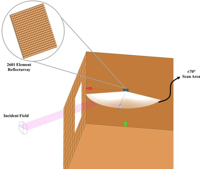
Fig. 6. Application case where the reflectarray redirects the incoming plane wave (incidence angle of the plane wave is at  $\theta = 20^\circ$ ) to the intended reception area.
