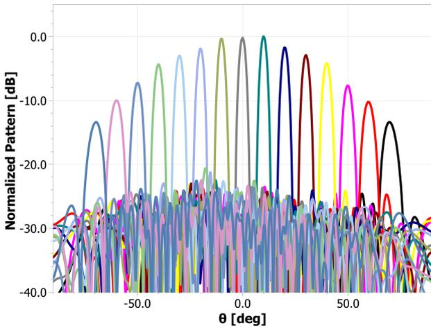
Fig. 8. Far-field radiation pattern of the optimised reflectarrays for scanned beams between  $\theta = \pm 70^\circ$ . (All beams have been optimized for 26 GHz)
