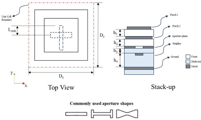
Fig. 1. Aperture coupled stacked patch element.
