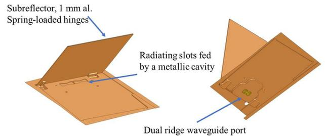
Fig. 5. Feed model of the cavity backed radiating slot antenna with planar subreflector.
