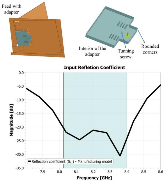
Fig. 9. Manufacturing model and input reflection coefficient after final optimization.
