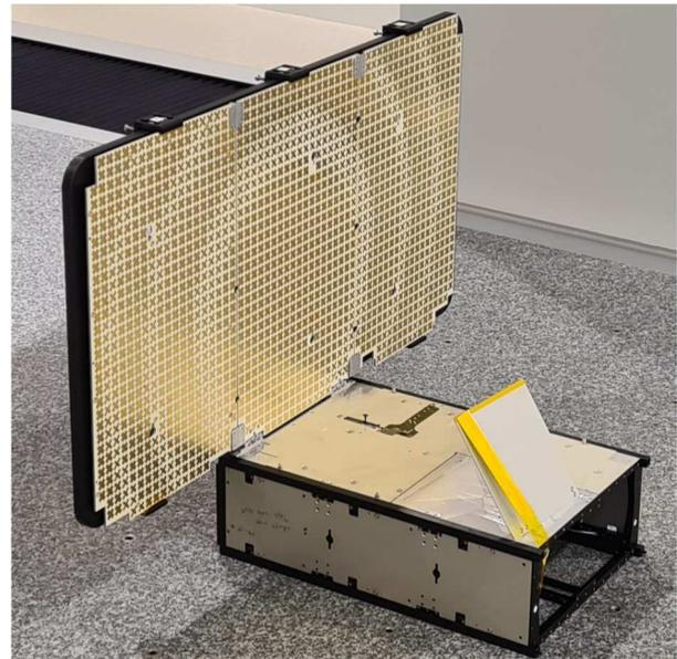
Fig. 1. Realized X-band polarizing reflectarray antenna system designed for 6U CubeSat platforms.
