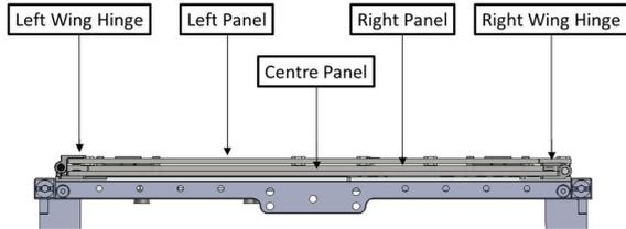
Fig. 2. CAD model of deployed antenna system.
