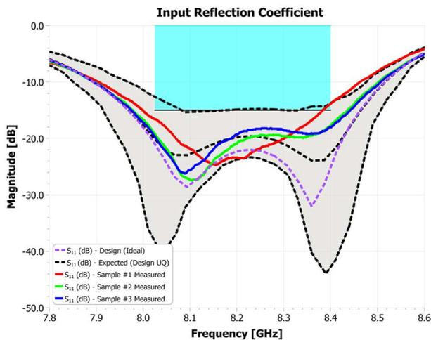
Fig. 14. Measured input reflection coefficients and calculated uncertainty intervals.
