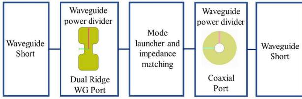
Fig. 6. Adapter topology block diagram.
