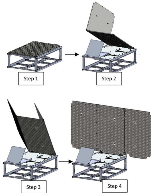
Fig. 2. Antenna system deployment sequence.
