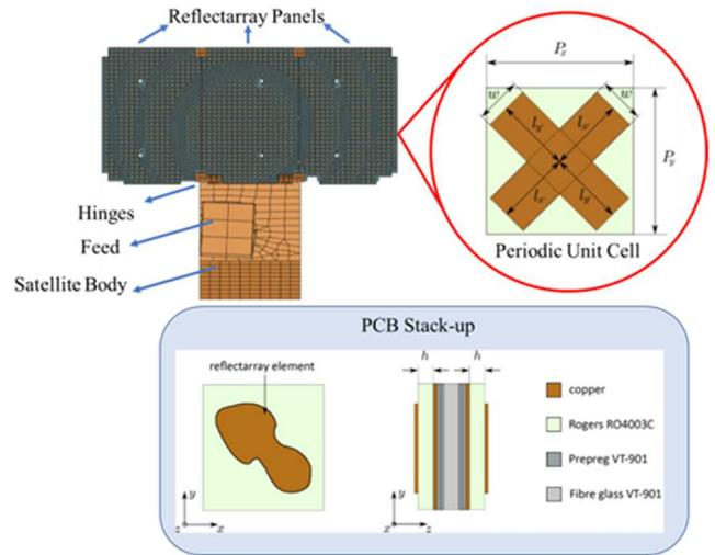
Fig. 4. Reflectarray antenna system model and periodic unit cell.
