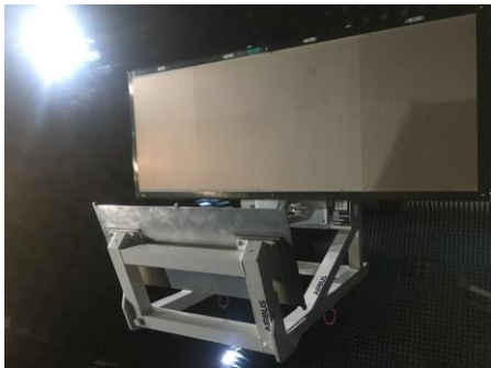
Fig. 3. Reflectarray breadboard in the AIRBUS Madrid anechoic chamber.
