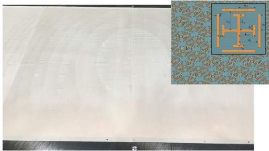
Fig. 2. Reflectarray panel and unit cell model used in the optimisation.
