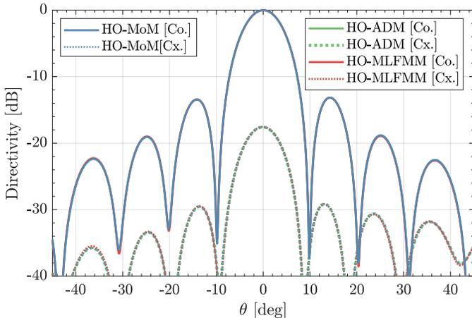
Fig. 2. Normalized far-field directivity pattern ( $\phi = 0^\circ$ -cut) for the sub-array in Fig. 1 at 8.425 GHz, comparing the extended HO-ADM to HO-MLFMM and HO-MoM. Co-polarization is RHCP whereas the cross-polarization is LHCP.
