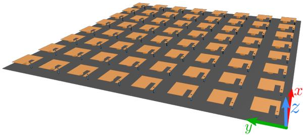
Fig. 1.  $8 \times 8$ -element (area of  $28.5\lambda^2$ ) dual-frequency right-hand circularly polarized (RHCP) high-gain antenna sub-array from [9], with radiation pattern coordinate system.
