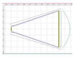
thorough design developments. S-parameters and return loss are typically considered in CHAMP 3D, just as the feed radiation may be formed to meet a specific pattern template. Rotationally symmetric terminals with one or two reflectors can be made to meet pattern constraints, e.g. sidelobe roll-off.
