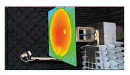
This procedure helps engineers to accurately reconstruct the extreme near field and surface currents of an AUT from the radiated field measured in anechoic chambers. Inspection of the extreme near field and currents allows quick identification of electrical or mechanical errors in the antenna, which cause anomalies in the measured field, saving valuable time and resources in the antenna design and validation process.
