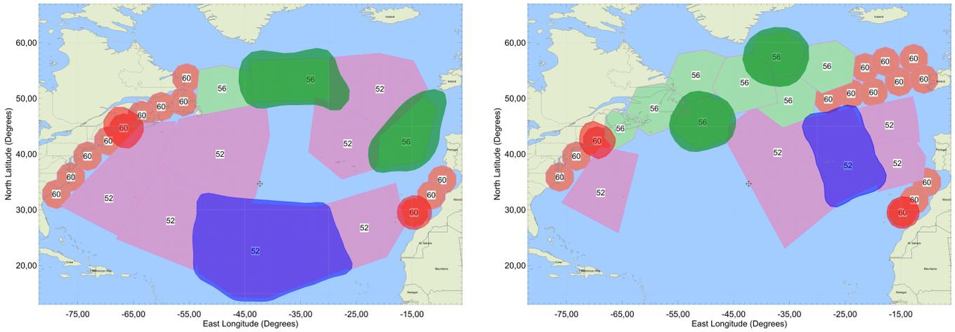
Fig. 4. The optimized radiation pattern of five of the beams in each coverage scenario plotted over the coverage polygons. The left figure is the 00:00UTC scenario and the right is the 12:00UTC scenario. Within the filled blue contours the EIRP is above 52 dB W, within the green EIRP is above 56 dB W, and within the red EIRP is above 60 dB W.
