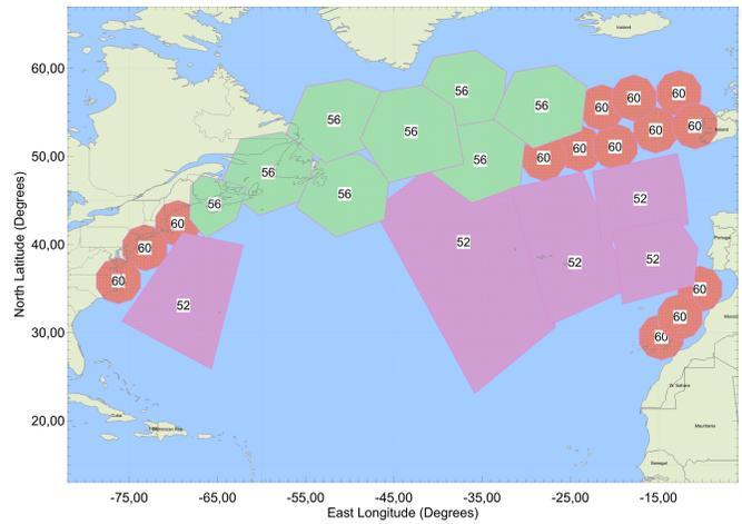
Fig. 2. Top row: Flight traffic over the Atlantic 12 hours apart (00:00UTC and 12:00UTC) on the 28th of April, 2022. Obtained from flightradar24.com. Bottom row: Coverage polygons for beams to service the 00:00UTC and 12:00UTC situations, respectively. Small beams (red) are designated an edge of coverage goal EIRP of 60 dB W, medium sized beams (green) 56 dB W, and large beams (purple) 52 dB W.
