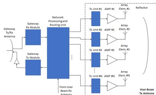
Fig. 1. Typical payload configuration for a digital payload using array-fed reflectors for the user beams. Only the Tx User Beam Antenna is included in this schematic. The User Beam Rx Antenna is assumed to be a separate array-fed reflector antenna with a set of Rx units.
