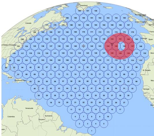
Fig. 3. Nominal beam directions corresponding to each of the 198 feeds and the defocused beam pattern of the 145th element.
