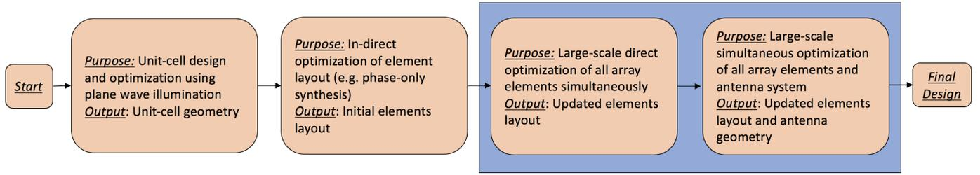
Fig. 1. Design procedure for the design of reflectarrays. The steps in the blue box are unique capabilities introduced in the design framework presented in this paper. The initial steps in the design process are identical to the existing design methods.
