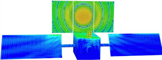
Fig. 5. Reflectarray model on ESA's M-ARGO CubeSat.
