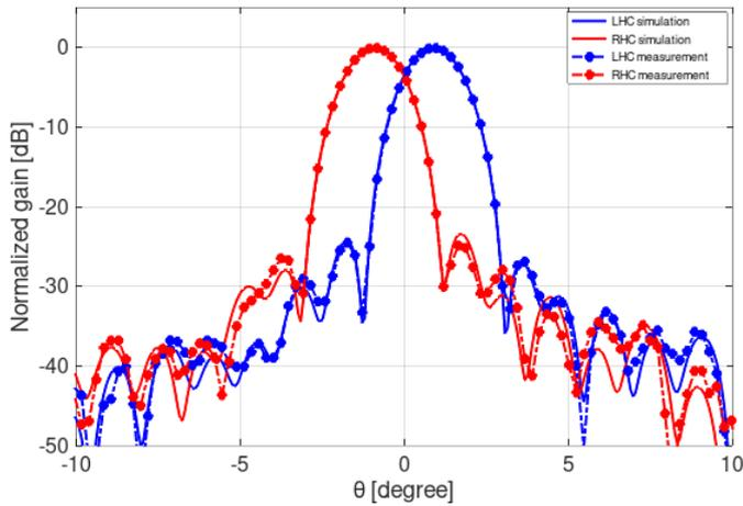
Fig. 4. Comparison of predictions and measurements of beams in the Tx band (18.8 GHz) of the doubly-curved linear-to-circular polarization reflectarray.
