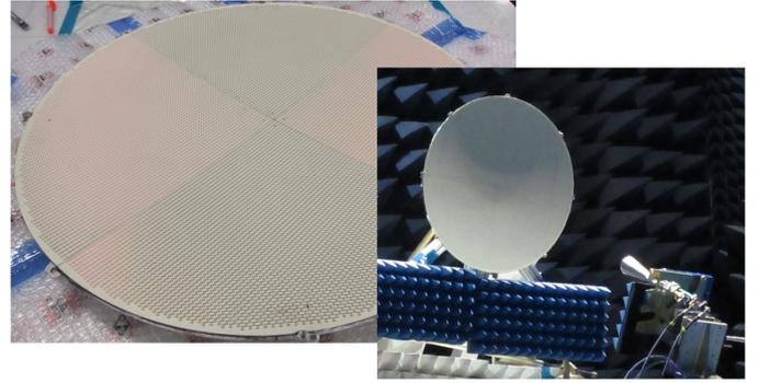
Fig. 3. Ka-band Tx/Rx curved multiple spot beam reflectarray.
