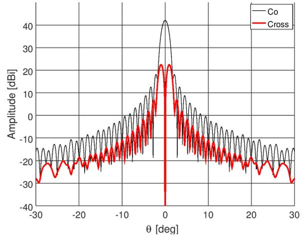
Fig. 3. The co- and cross polarization radiation patterns in the 90 degree plane when the feed is excited by the fundamental  $TE_{11}$  mode.
