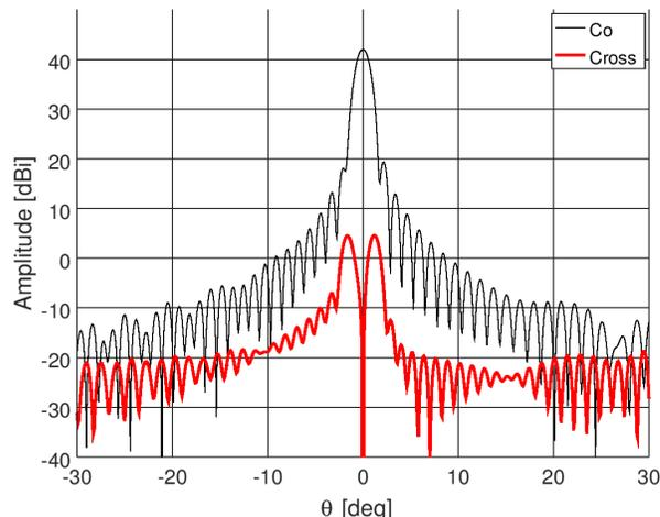
Fig. 6. The co- and cross polarization radiation patterns in the plane of maximum cross polarization ( $\phi = 45$  degrees) after a direct optimization of the mode converter with minimum cross polarization level in the secondary pattern as goal.
