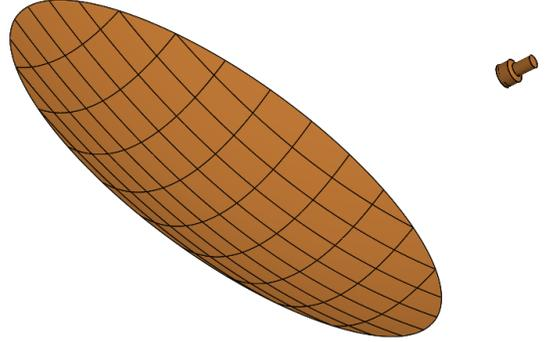
Fig. 2. The considered offset reflector configuration in which the feed is a corrugated horn.
