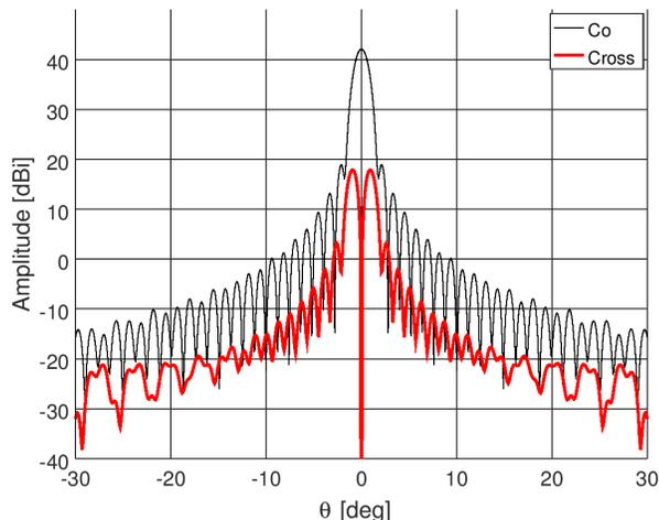
Fig. 5. The co- and cross polarization radiation patterns in the plane of maximum cross polarization ( $\phi = 90$  degrees) after the mode converter is optimized for the scattering parameter ratio in (1).
