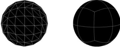
Fig. 1. Meshing of a sphere. Left: Lower-order flat triangular patches. Right: Higher-order, curved quadrilaterals.
