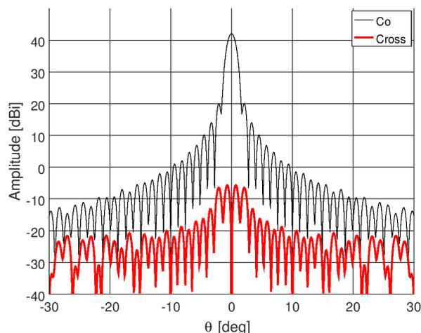
Fig. 7. The co- and cross polarization radiation patterns in the plane of maximum cross polarization ( $\phi = 90$  degrees) after a direct optimization of the mode converter as well as the first four horn corrugations with minimum cross polarization level in the secondary pattern as goal.
