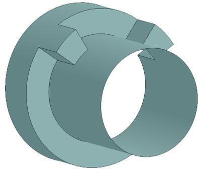
Fig. 4. The mode converter generating the higher-order  $TE_{21}$  mode. The length of the grooves as well as the mode converter length are optimized.
