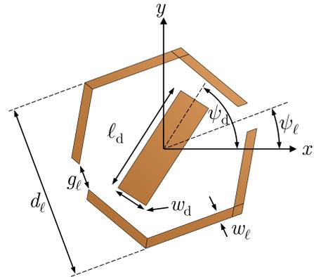
Fig. 2. Split hexagonal-loop dipole element.
