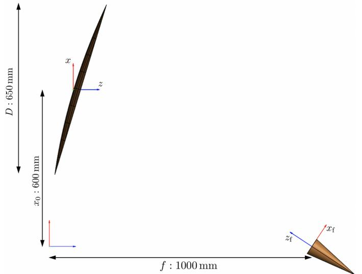
Fig. 1. Reflectarray configuration. The  $xyz$ -coordinate system represents the reflectarray coordinate system and the  $x_f y_f z_f$ -coordinate system the feed coordinate system.
