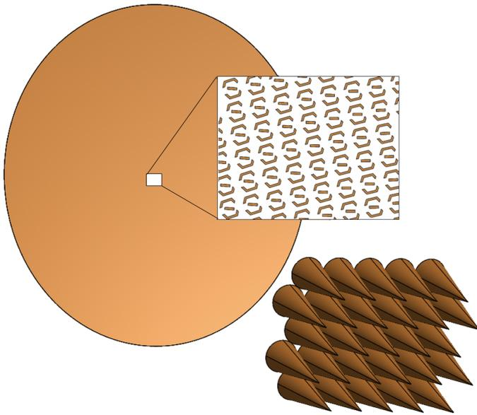
Fig. 4. Reflectarray illuminated by a feedarray consisting of 27 feeds in a hexagonal grid.
