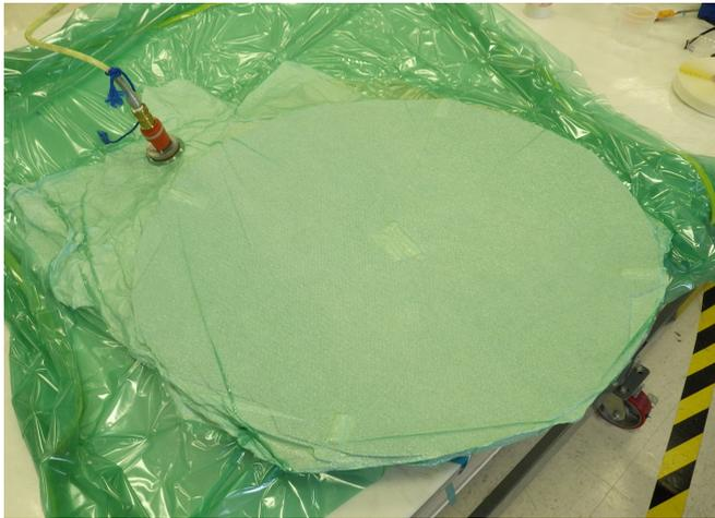
Fig. 6. Vacuum bagged reflector mold assembly during ambient curing.
