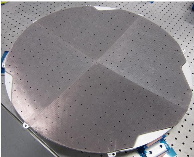
Fig. 7. Conformed test pie slices bonded to the aluminum reflector mold.
