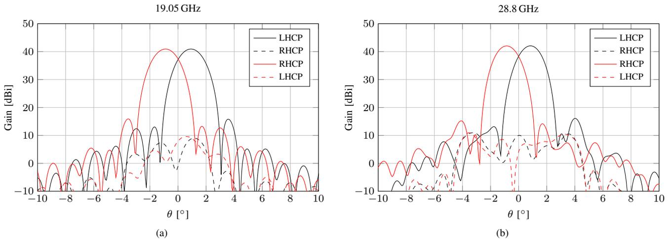
Fig. 3. Radiation pattern of Tx and Rx beams when illuminated by LHCP (black) and RHCP (red) incident field with the feed in the focal point at the center Tx/Rx frequencies. The  $\phi = 90^\circ$  cut is shown, i.e., the cut orthogonal to the offset plane.
