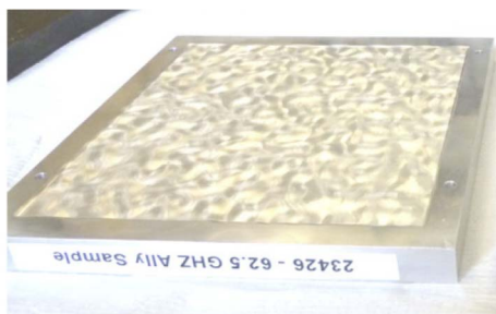
Fig. 3. Manufactured rough aluminum sample: roughness of Gaussian distribution with correlation length of 3.86 mm and rms of 0.1 mm.
