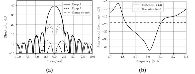
Fig. 5. Cross-polar performance of the  $TM_{01}$  matched feed. (a): Reflector radiation pattern in asymmetry and diagonal planes. Cross polarization of a Gaussian beam feed is indicated in grey. (b): Cross polarization relative to peak directivity as a function of frequency.
