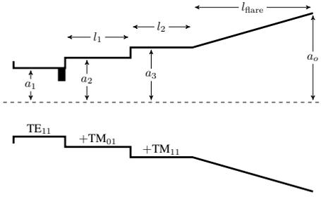
Fig. 3. Topology of the  $TM_{01}$  matched feed. The pin type mode launcher is indicated in the step between  $a_1$  and  $a_2$ .
