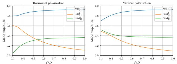
Fig. 1. Optimized mode excitation coefficients for  $f/D$  values between 0.3 and 1.  $TE_{21}$  modes have been excluded.
