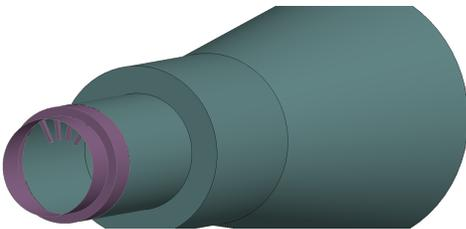
Fig. 4. Feed viewed from the back. The  $TM_{01}$  mode launcher part is highlighted showing the four radial pins.
