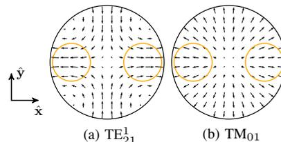
Fig. 2. Transverse fields of the  $TE_{21}^1$  and the  $TM_{01}$  mode. The equivalent regions of cross polarization equivalent are highlighted.
