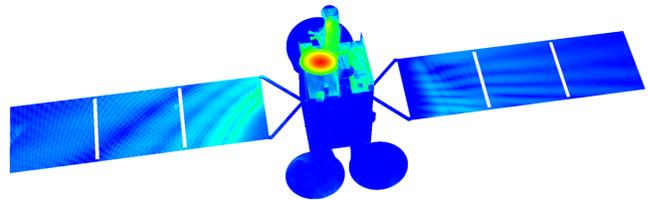
Fig. 3. Currents on the satellite platform computed with Higher-Order MLFMM at Q-band (40 GHz).
