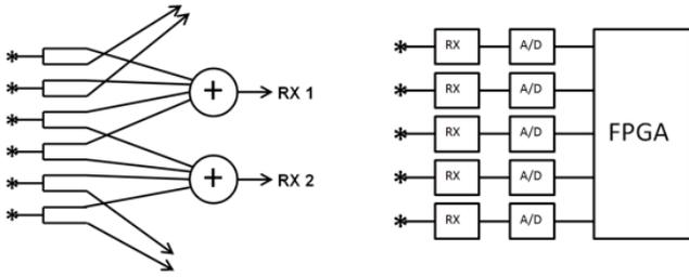
Fig. 4. Dense array receiver system
