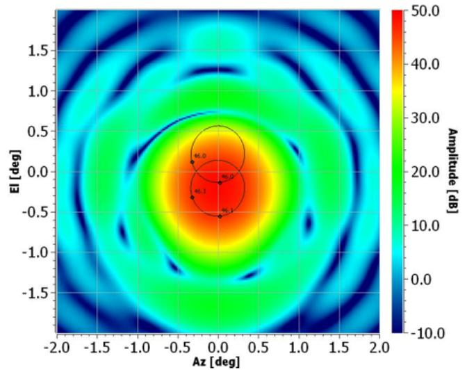
Fig. 6. C-band FPA makes 2 beams with suitable overlap
