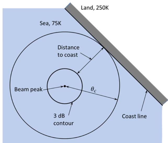
Fig. 1. Schematic of the distance to coast issue
