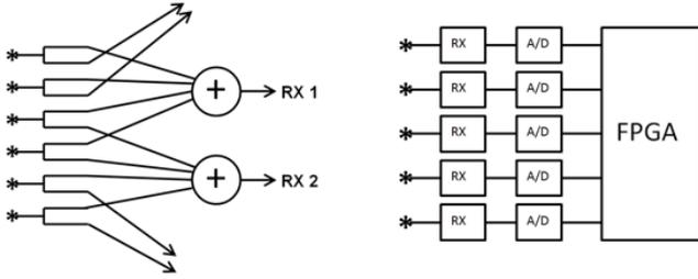
Fig. 4. Dense array receiver system
