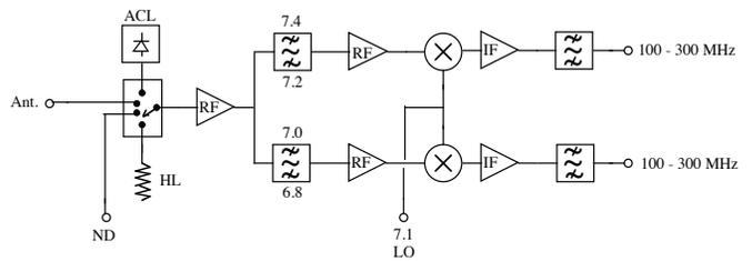
Fig. 7. Dual frequency C-band receiver
