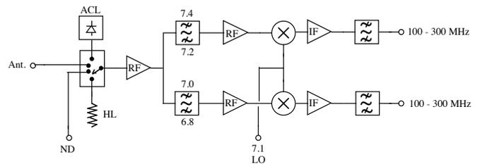
Fig. 7. Dual frequency C-band receiver
