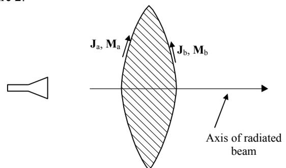
Figure 2: Equivalent currents on lens.
