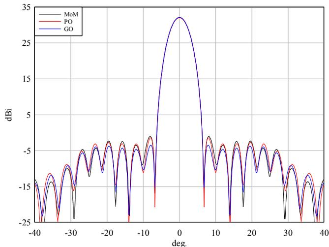
Figure 8: Comparison of MoM, PO and GO for  $D=15\lambda$ .
