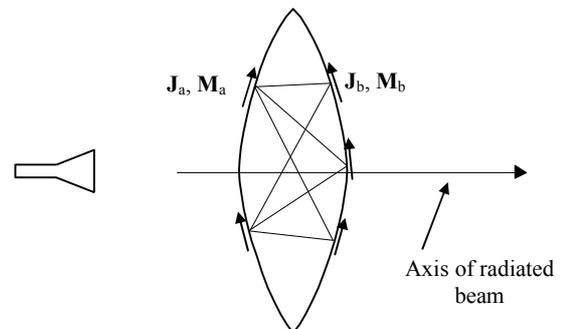
Figure 4: PO lens calculation. All currents in the integration points on the left hand surface radiate through the lens material to the integration points on the right hand surface.
