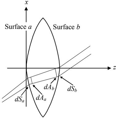
Figure 5: GO lens calculation. The power is conserved in the ray tube inside the lens.
