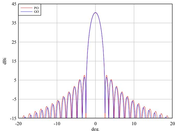
Figure 9: Comparison of PO and GO for  $D=40\lambda$ .
