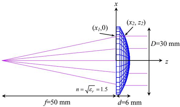
Figure 6: Plano-convex lens that transforms a spherical wave into a plane wave.
