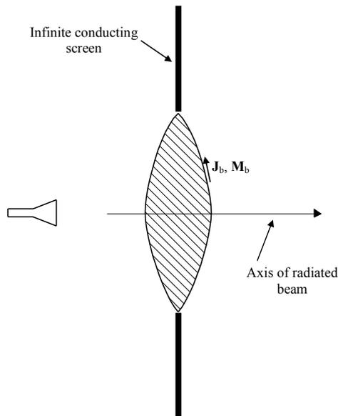
Figure 3: Lens mounted in an infinite conducting screen.
