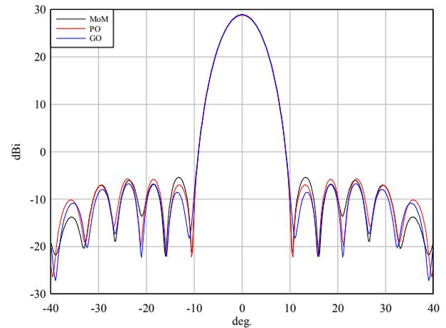
Figure 7: Comparison of MoM, PO and GO for  $D=10\lambda$ .
