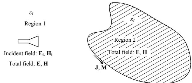
Figure 1: Equivalent currents on dielectric object.
