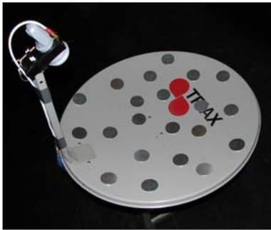
**Figure 14. Offset reflector with surface distortions.**
