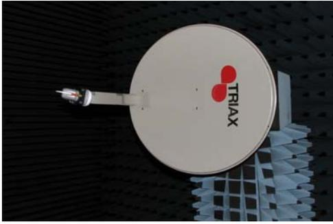
**Figure 8. Offset reflector with a feed tilt.**
