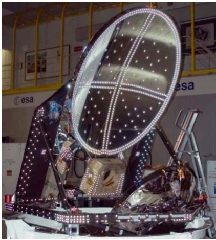
Fig. 1 The Planck telescope, prior to integration and without the horns of the focal plane. The white dots are the photogrammetry targets, which were removed before integration of the telescope into the satellite. Figure courtesy of ESA and Thales Alenia Space France.
