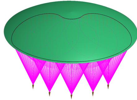
Fig. 3. Rim trace for toroidal push-broom antenna design.
