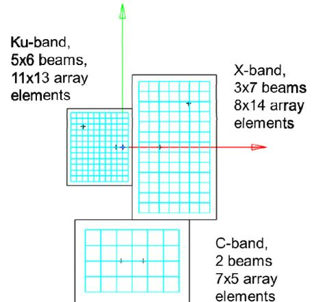
Fig. 5. Feed arrays located in the focal plane.
