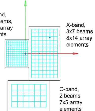
Fig. 5. Feed arrays located in the focal plane.
