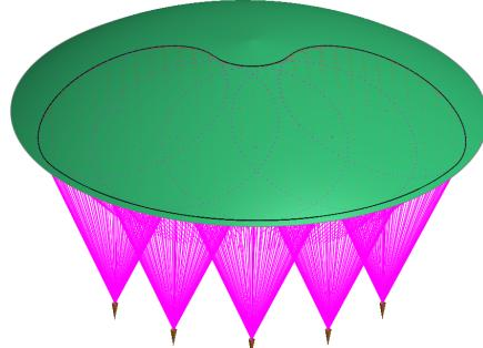
Fig. 3. Rim trace for toroidal push-broom antenna design.
