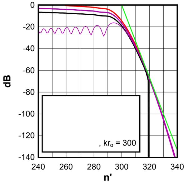
**Figure 9** The truncated power  $P_{tr}^{(n)}$  scaled in  $n$ , for Hertzian dipoles at  $kr_o = 30, 300$  and  $3000$  and the power spectrum  $P_{rad}^{(n)}$  for  $kr_o = 300$ .
