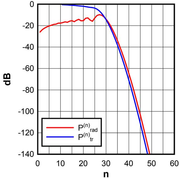
Figure 3 Power spectrum  $P_{rad}^{(n)}$  and truncated power  $P_{tr}^{(n)}$  for a  $\hat{z}$ -directed Hertzian dipole at  $kr_o = 30$ .
