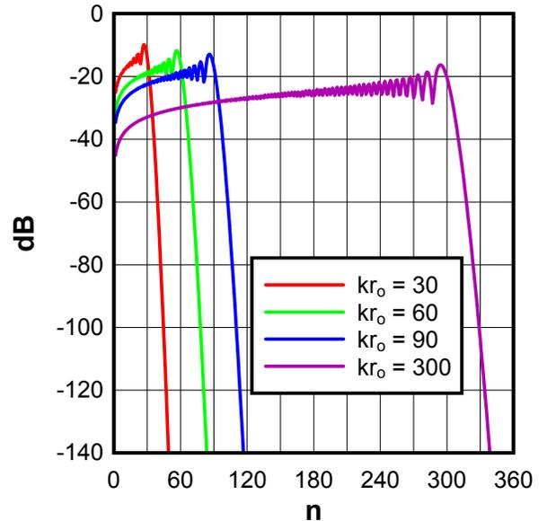
Figure 5 Power spectrum  $P_{rad}^{(n)}$  for Hertzian dipoles at different positions  $r_o$ .
