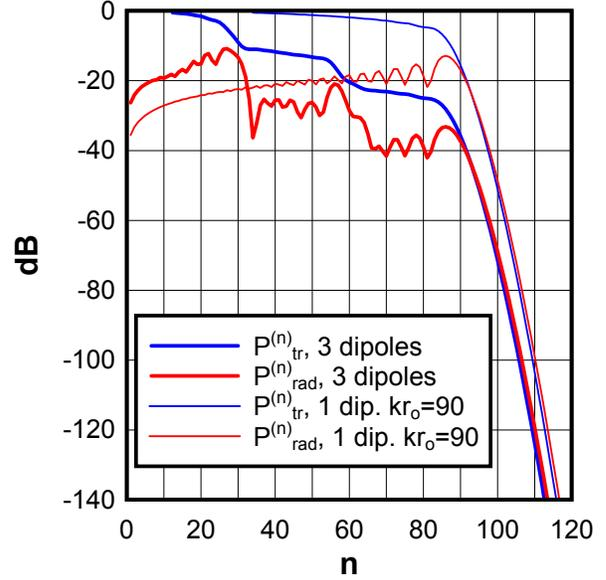
**Figure 10** Truncated power  $P_{tr}^{(n)}$  and power spectrum  $P_{rad}^{(n)}$  for an array of three Hertzian dipoles compared to those for the outermost dipole alone.
