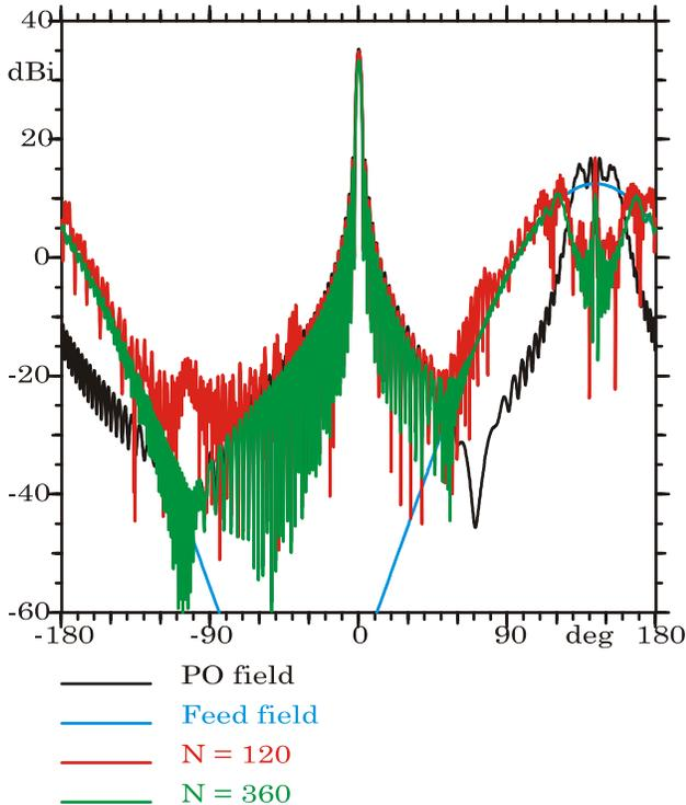
Figure 12 Patterns of the off-set reflector antenna.
