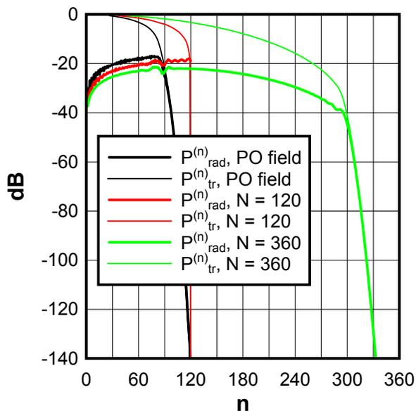
Figure 13 Mode spectra of the reflector antenna and of the reflector PO field alone.
