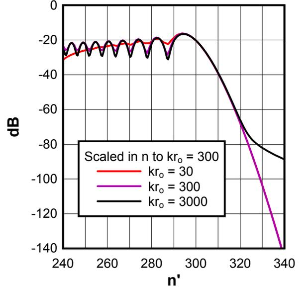
**Figure 7** Part of the power spectra, scaled in  $n$ , for Hertzian dipoles at  $kr_0 = 30, 300$  and  $3000$ . The last case is inaccurate below -70 dB.
