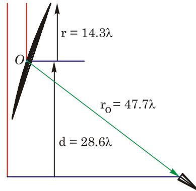
**Figure 11** Off-set reflector antenna.
