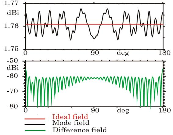
Figure 4 The far field for  $\theta = 90^\circ$  of the  $\hat{z}$ -directed dipole at  $kr_o = 30$ . Top: ideal field and field based on  $N = 40$  modes. Bottom: difference field with 41 lobes.
