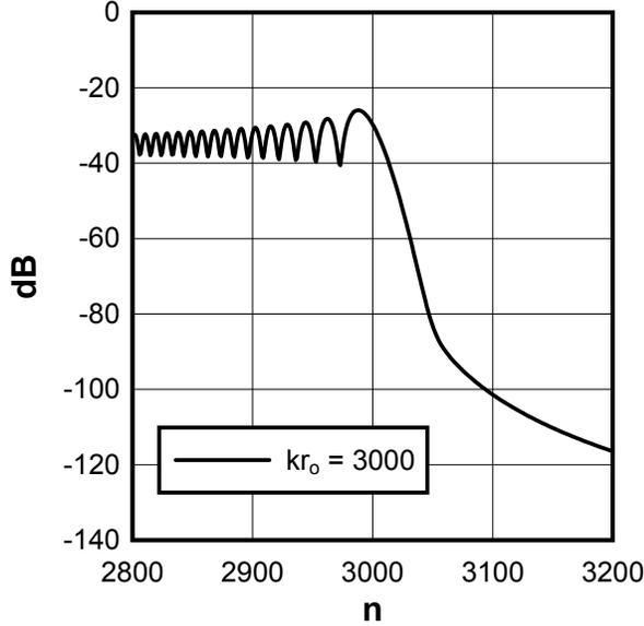
**Figure 6** Part of the power spectrum  $P_{rad}^{(n)}$  for a Hertzian dipole at  $kr_0 = 3000$ .
