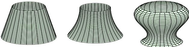
Fig. 1. Surfaces realized using a single BoR patch of first (left), second (centre), and third order (right), respectively. The generatrix is described by a Lagrange polynomial passing through 2, 3, or 4 interpolation nodes, respectively. The cubic patches using 4 interpolation nodes per patch generally provides the highest accuracy for curved surfaces and is preferred for reflectors.
