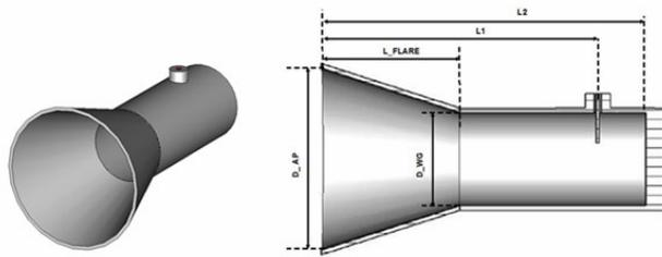
Fig. 3 Geometry of the feeder
