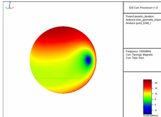
Fig. 6 First iteration. Equivalent magnetic currents [dBV/m]
