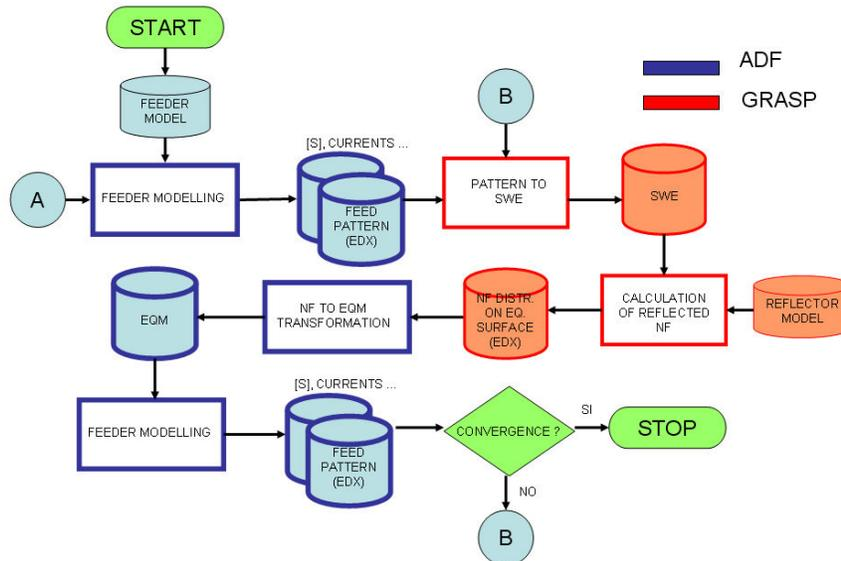
Fig. 2 Flow chart of the iterative procedure
