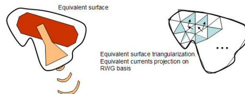
Fig. 1 Application of the equivalence theorem
