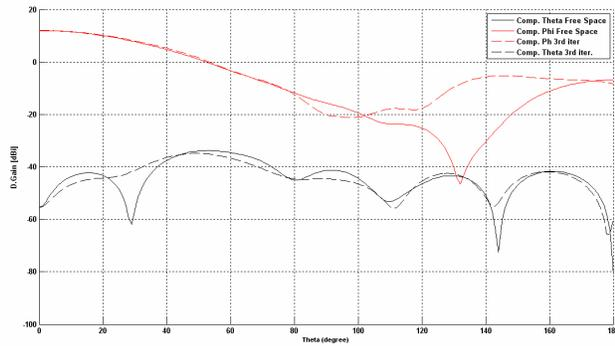
Fig. 8 Final iteration. Feeder directivity gain [dBi]
