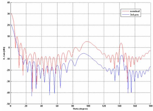
Fig. 10 Full-wave results. Reflector directivity gain [dBi]
