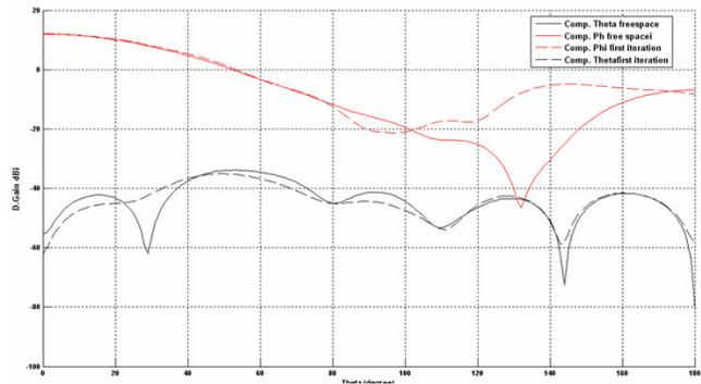
Fig. 7 First iteration. Feeder directivity gain [dBi]
