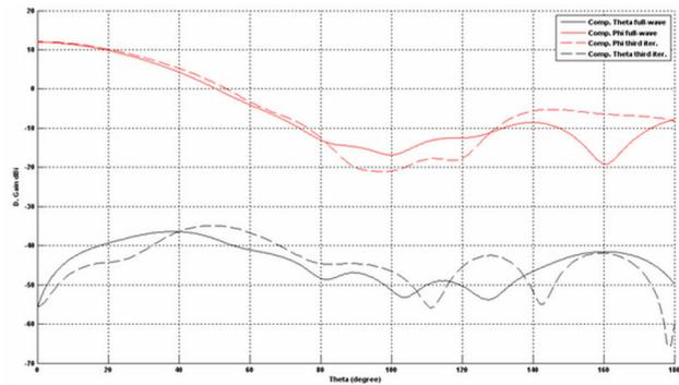
Fig. 11 Full-wave results vs. iterative method results. Feeder directivity gain [dBi].  $\Phi = 0^\circ, \Theta = 0^\circ, 180^\circ$ .
