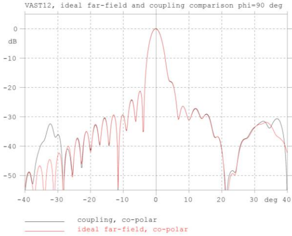
Fig. 7 – Amplitude of the far-field and coupling pattern for a uniform CATR distribution and the VAST12 antenna.
