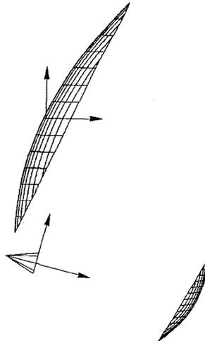
*Figure 1. Geometry of shaped dual offset reflector for rectangular coverage. The original system is designed to 9.2° by 4.6°, and the subreflector is re-shaped to an enlarged coverage of 11.9° by 4.6°.*
