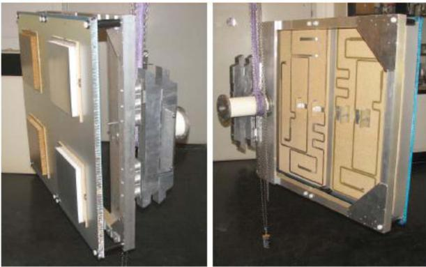
Figure 2. The feed array and its support structure.
