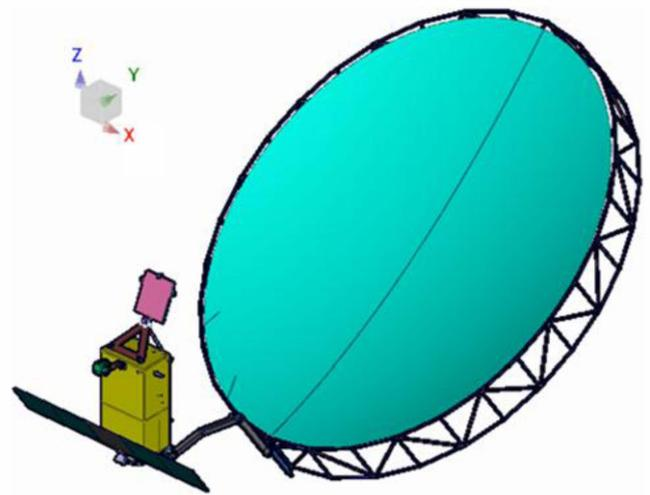
Figure 1. The feed array (in pink), the satellite body (in yellow) and the large deployable reflector (in blue).
