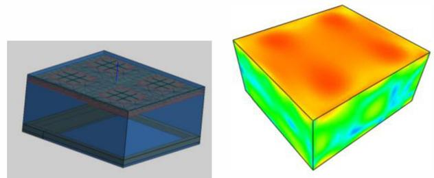
Figure 5. The feed array and the support structure of configuration B, together with the reconstruction surface (a blue box enclosing the antenna), on the left. The amplitude of the total electrical currents computed by DIATOOL, for configuration B.
