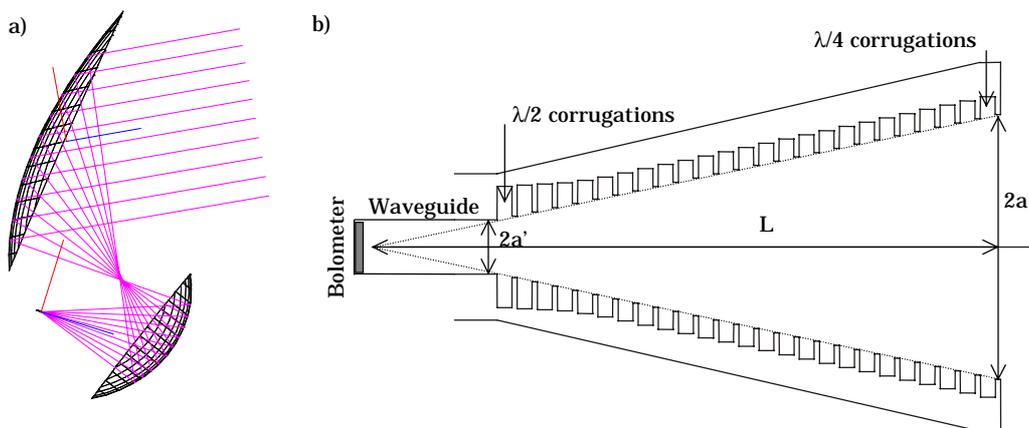
**Figure 1** In a) the Planck telescope is illustrated. The telescope is an aplanatic system consisting of two ellipsoidal reflectors, the main reflector having a diameter of 1.5 m. Operating at 857 GHz the feed horns are placed slightly out of focus. In b) a drawing of a standard corrugated horn that employs a bolometric detector is shown.
