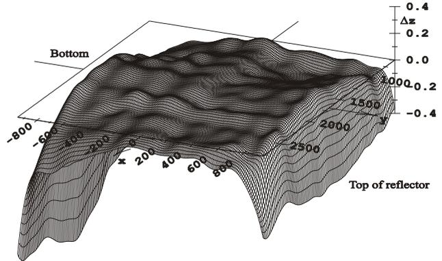
**Figure 10 – Subreflector. Deviation ( $\Delta z$ , positive towards the feed) of the interpolated measured surface from the best-fit parabolic surface. All measures are in mm.**
