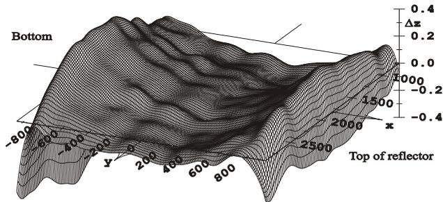
**Figure 9 – Subreflector. Deviation ( $\Delta z$ , positive towards the feed) of the interpolated measured surface from the best-fit parabolic surface. All measures are in mm.**
