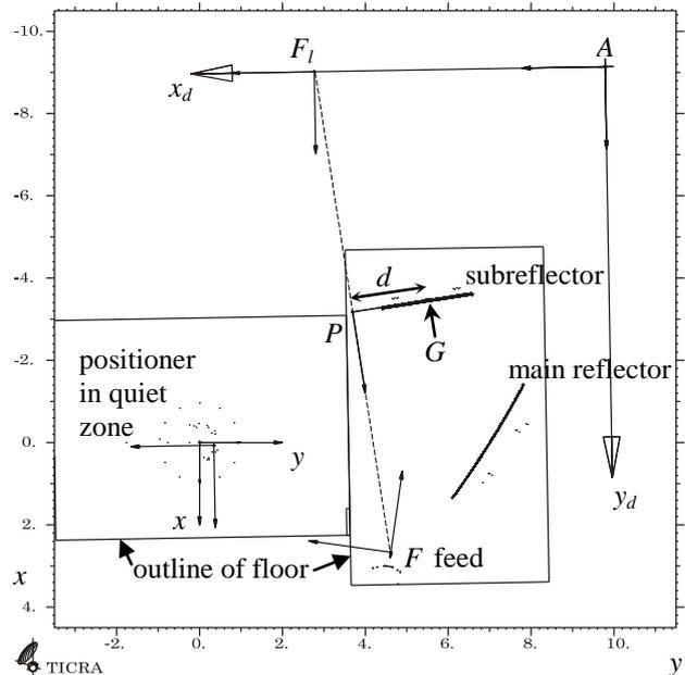
**Figure 4 – The geometry of the CATR before relocation given by the points sampled by the laser tracker. The outline of the floor is illustrated by two rectangles.**
