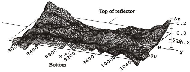
**Figure 8 – Main reflector. Deviation ( $\Delta z$ , positive towards the quiet zone) of the interpolated measured surface from the best-fit parabolic surface. All measures are in mm.**
