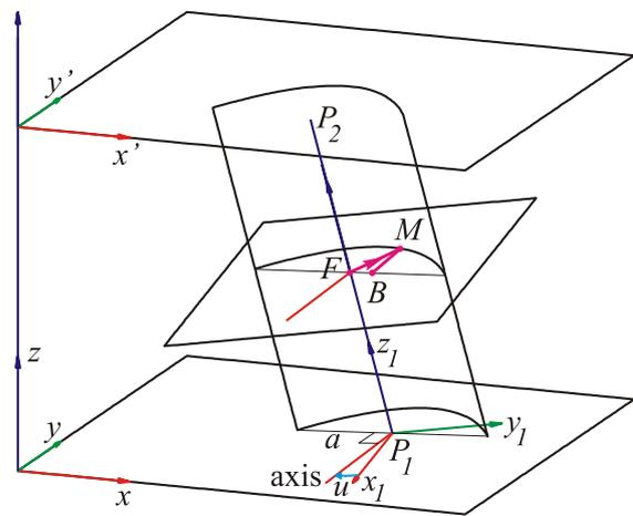
**Figure 6 – Determination of the best-fit main reflector.  $P_1P_2$  is the focal line and the aperture plane is spanned by this focal line and the line  $a$ . The primed coordinates are parallel to the corresponding unprimed.**
