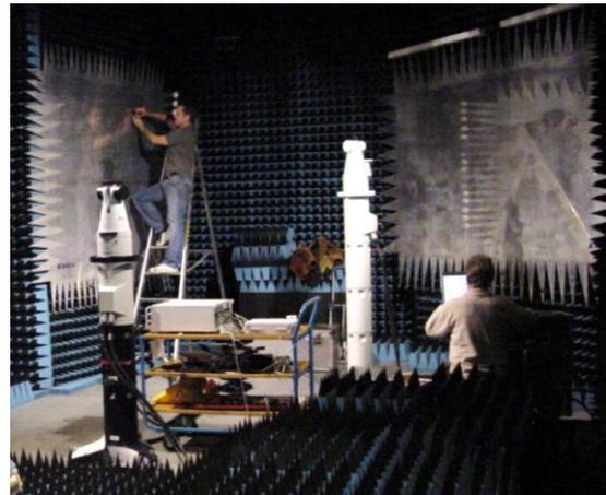
**Figure 11 – Sampling the surface of the relocated subreflector by laser tracking of a hand-held target.**
