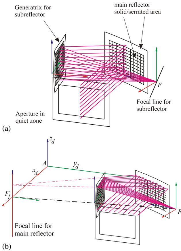
**Figure 2 – Illustration of the singly curved double reflector range. The GO rays are collimated vertically by the subreflector (a) and horizontally by the main reflector (b).**
