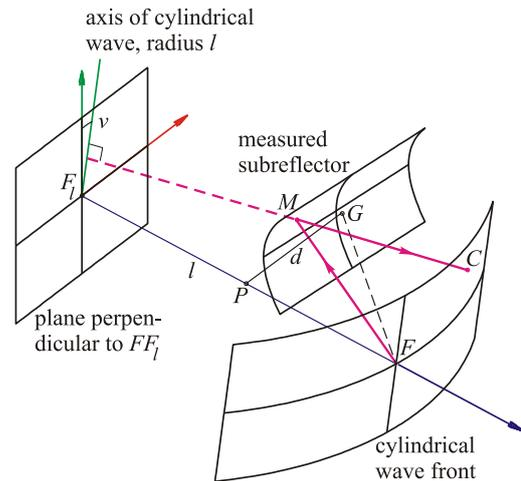
**Figure 7 – Determination of the best-fit subreflector. Ray  $FMC$  equals  $l$  for the ideal surface.**
