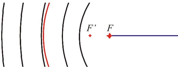
**Figure 5 – Parabolas with focal point at  $F$  and different focal lengths (black). The parabola which fits best to a measured parabola (red) requires the focal point to be moved to  $F'$ .**
