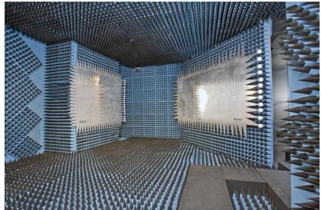
**Figure 1 – The CATR after relocation, main reflector to the right, subreflector to the left. The feed is hidden in a niche to the right behind foreground absorbers.**
