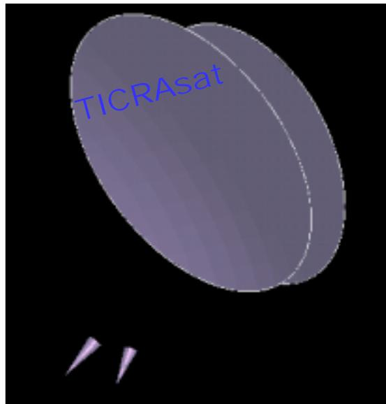
Fig.2 Interleaved reflectors in a dual-gridded system. The front reflector has metal strips deposited on a dielectric support shell, thus reflecting the majority of the field coming from one of the feeds, whereas the other feed field is transmitted through the front and reflected from the rear shell.
