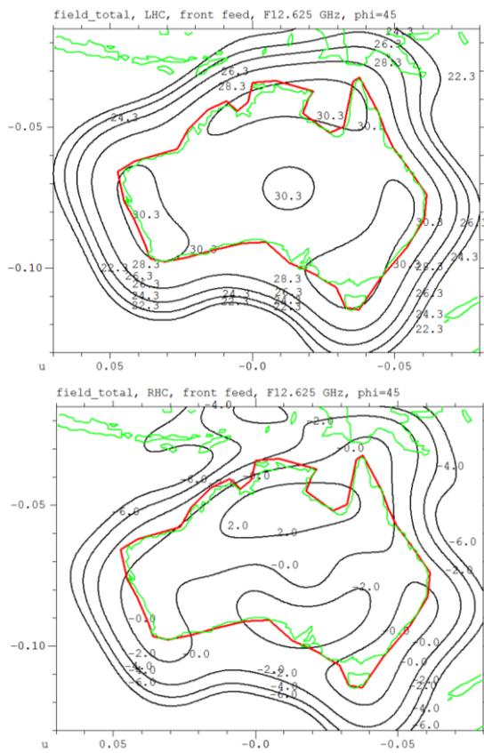
Fig. 6. Antenna patterns, total field, for the real CPSS reflectors at 12.625 GHz: LHCP coverage obtained from the LHCP front feed, CPSS orientation  $\phi=45$  deg. Above is the co-polar LHCP component, below the cross-polar RHCP component.
