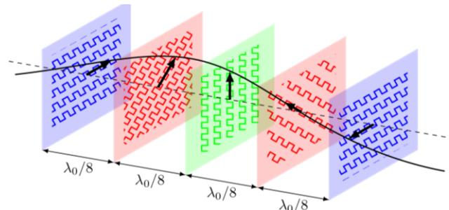
Fig. 2. Principal design of the CPSS. Metal meander line sheets separated by  $\lambda_0/8$  are rotated 45 degrees with respect to the neighboring sheet. The electric field of a LHCP wave has been indicated at each sheet. In the final design, the sheet separation and meander line parameters are optimized using full wave simulations.
