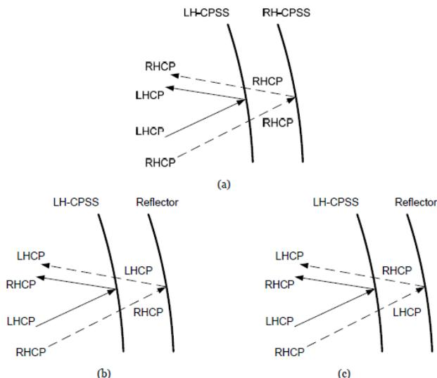
Fig. 1. Dual reflector CPSS geometries equivalent to DGR in CP: in (a) a reciprocal and symmetrical CPSS, in (b) a non-reciprocal and symmetric CPSS with a solid reflector and in (c) a non-reciprocal and asymmetric CPSS with a solid reflector.
