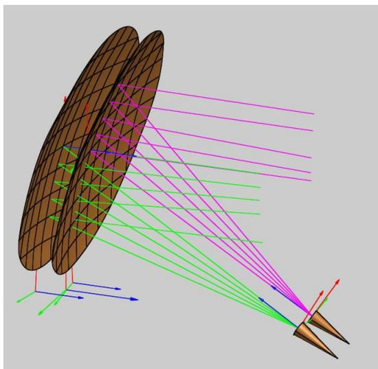
Fig. 4. The reciprocal CPSS reflector designed for the study: rays from the LHCP (in pink) and RCHCP (in green) feed are highlighted, as well as the rays reflected and transmitted by the CPSS surfaces.
