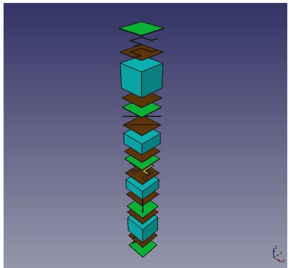
Fig. 3. Exploded view of the CPSS unit cell. Substrates are green, metal structures are yellow, bond films are brown, and spacers are cyan. The metal structures are embedded in the bond films, leaving an imprint.
