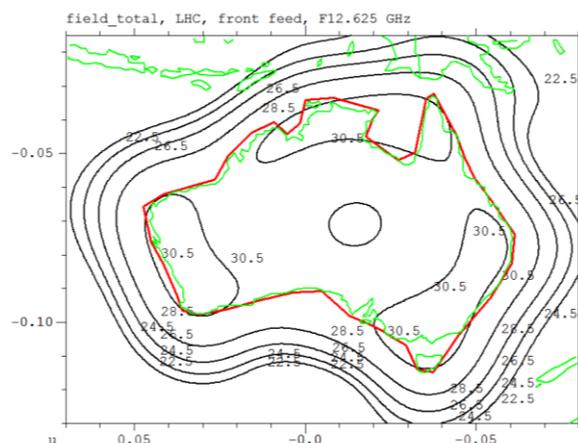
Fig. 5. Antenna pattern in dBi with ideal CPSS reflector surfaces at 12.625 GHz: LHCP coverage obtained from the LHCP front feed, the field is reflected in the front reflector, which is an ideal LH-CPSS.
