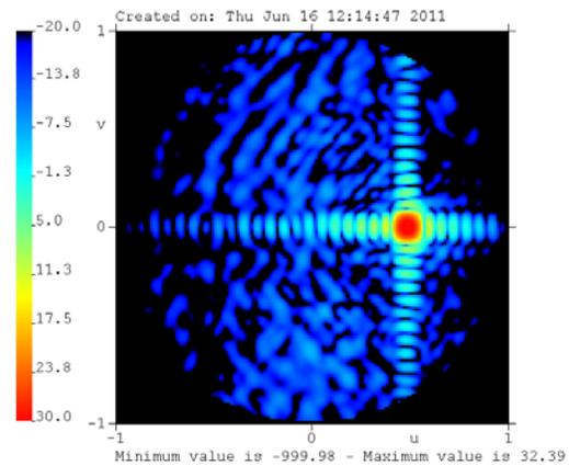
Figure 11 U-v pattern for optimized reflectarray example.
