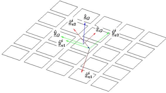
Figure 6. Skew angled coordinates for arbitrary incidence.
