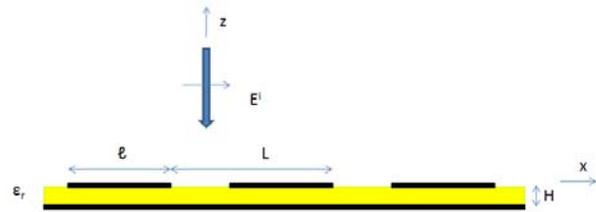
Figure 1. Strip array model of reflectarray.
