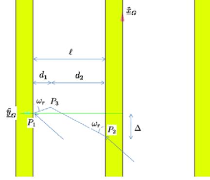
Figure 7. Determination of position of conducting walls.
