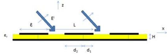
Figure 4 Strip array model of reflectarray.
