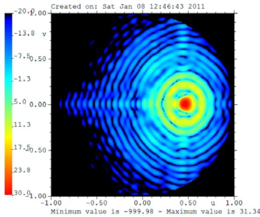
Figure 9 U-v pattern for reflectarray example.
