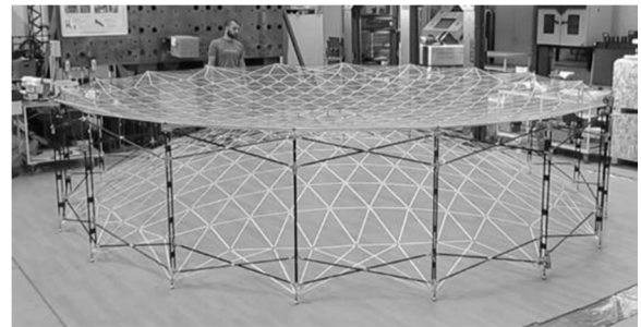
Figure 2. Double shifted Pantograph ring based crossed network technology demonstrator, ESA project SCALABLE, [9].
